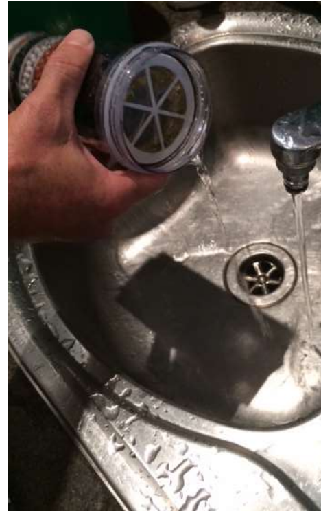
When filled tip out water. Repeat until water runs clean
