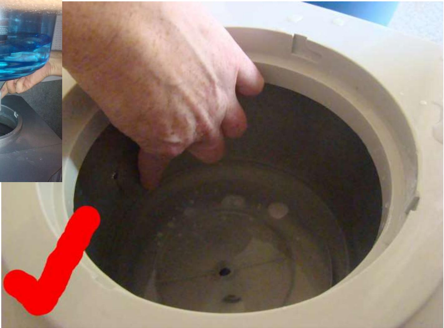
**Wait until the water has filled up bottom bowl, lift out the bowl from the base to check water level in tank. It should now only be half way full.**
