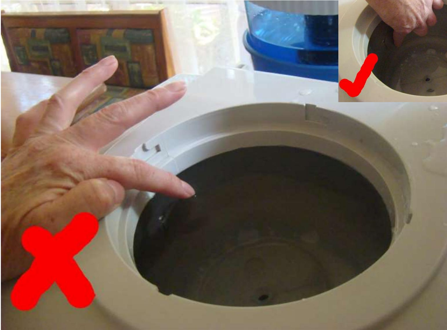
**If the water tank is more than half way full it means the float valve is not locking**
