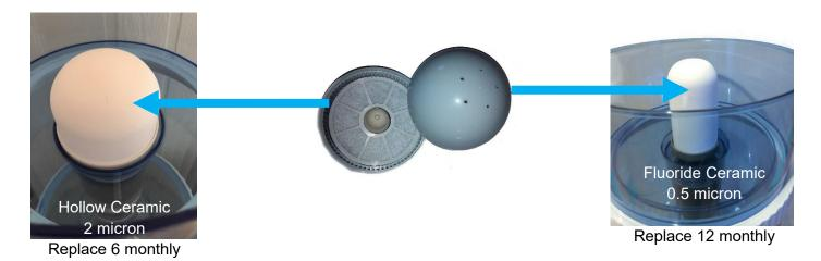
UNSCREW FILTER ANTI-CLICK WISE FROM BOTTOM BOWL. UNDO NUT AT THE UNDER THE BOTTOM BOWL TO REMOVE STANDARD DOME. REPLACE WITH CERAMIC DOME
