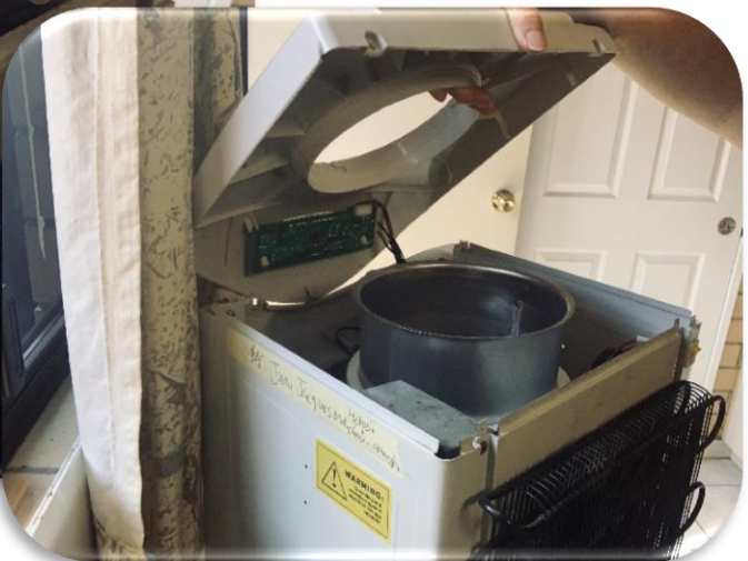
Lift top cover from the back as indicated here
