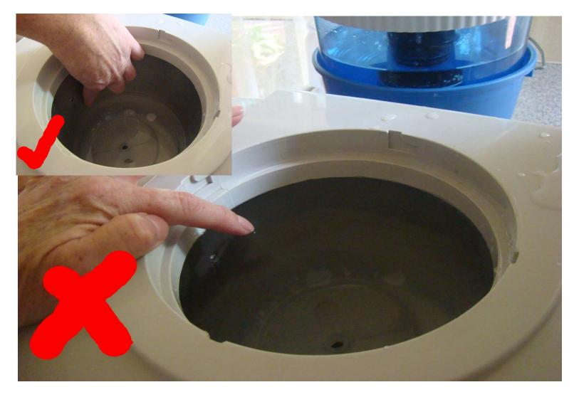
Lift the bottle part off the machine & place in a bucket. Check the water level in the tank. If the water tank is more than half way full it means the float value is not locking
