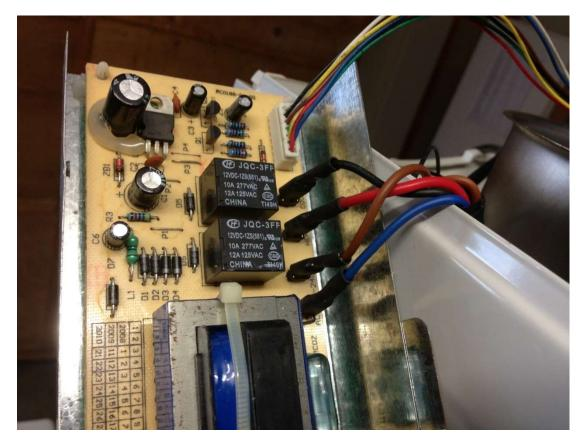
Check for any signs of damage (electrical burns) on the motherboard. If nothing on the front, undo the motherboard from the casing and check back. It is possible that only the section that controls the hot got damaged, but cold is still working.
