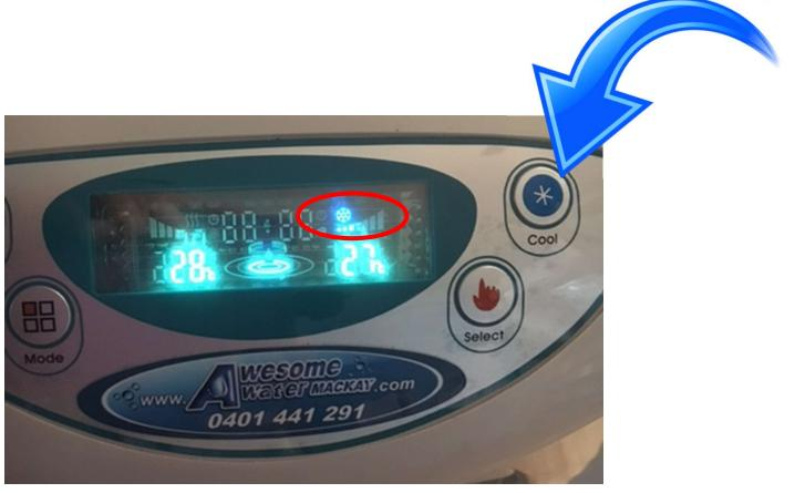
If the power trips when turning on the cold water it's either the motherboard that got damaged (see page 12) or the compressor has died. If the latter – this cannot be repaired.
