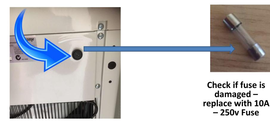
If there is no fuse casing on the back as indicated, the casing is internal – pre 2006 model and repair not recommended
