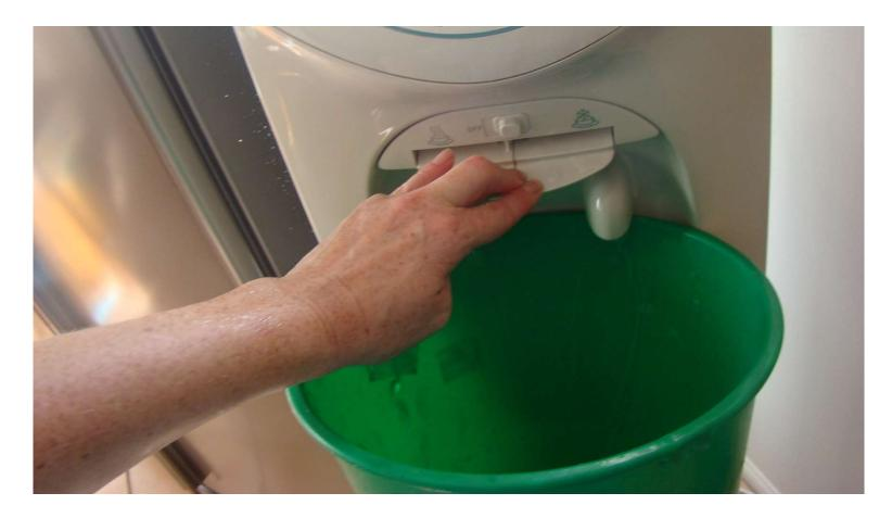
Drain the water in the tank by running both taps, until the tank is completely empty
