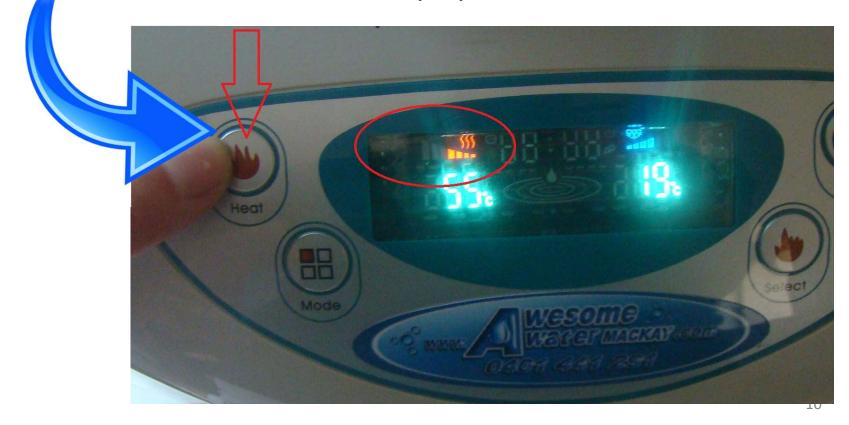
If the power trips when turning on the hot water, it could be either the hot relay on the **motherboard** that is damaged or the kettle element that has burned out.
