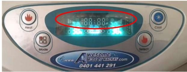
Turn cold water on by pushing the Cool button – top right once. The blue snowflake & blue bars will come on.
