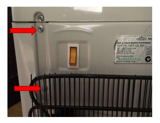
Undo metal box where motherboard is located by removing 2 x screws at back of machine that holds metal box in place.
