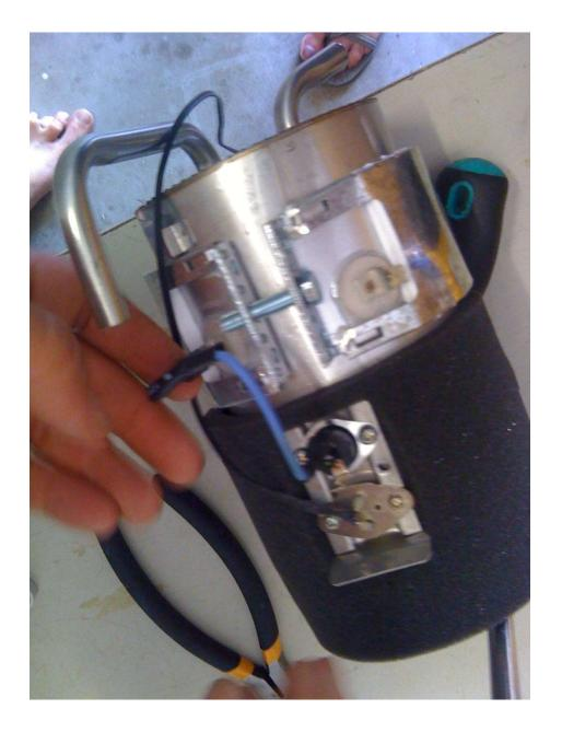
If the motherboard seems fine then it is most likely the kettle element that has burn out. The kettle will need to be replaced.
