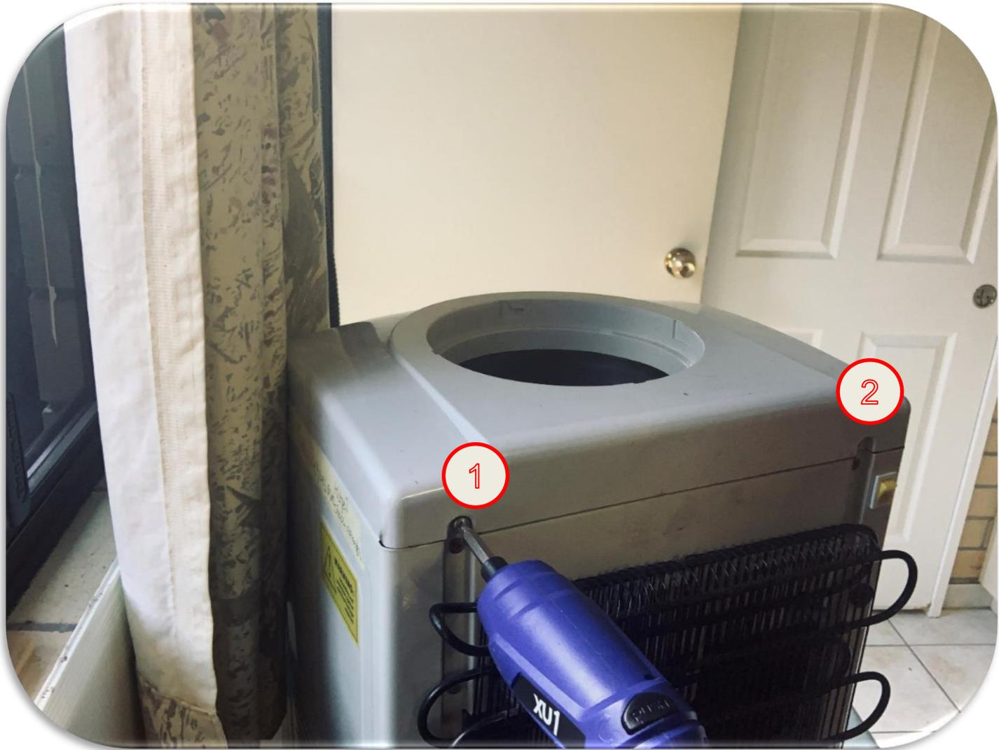
Unscrew 2 x top screws at back of the cooler
