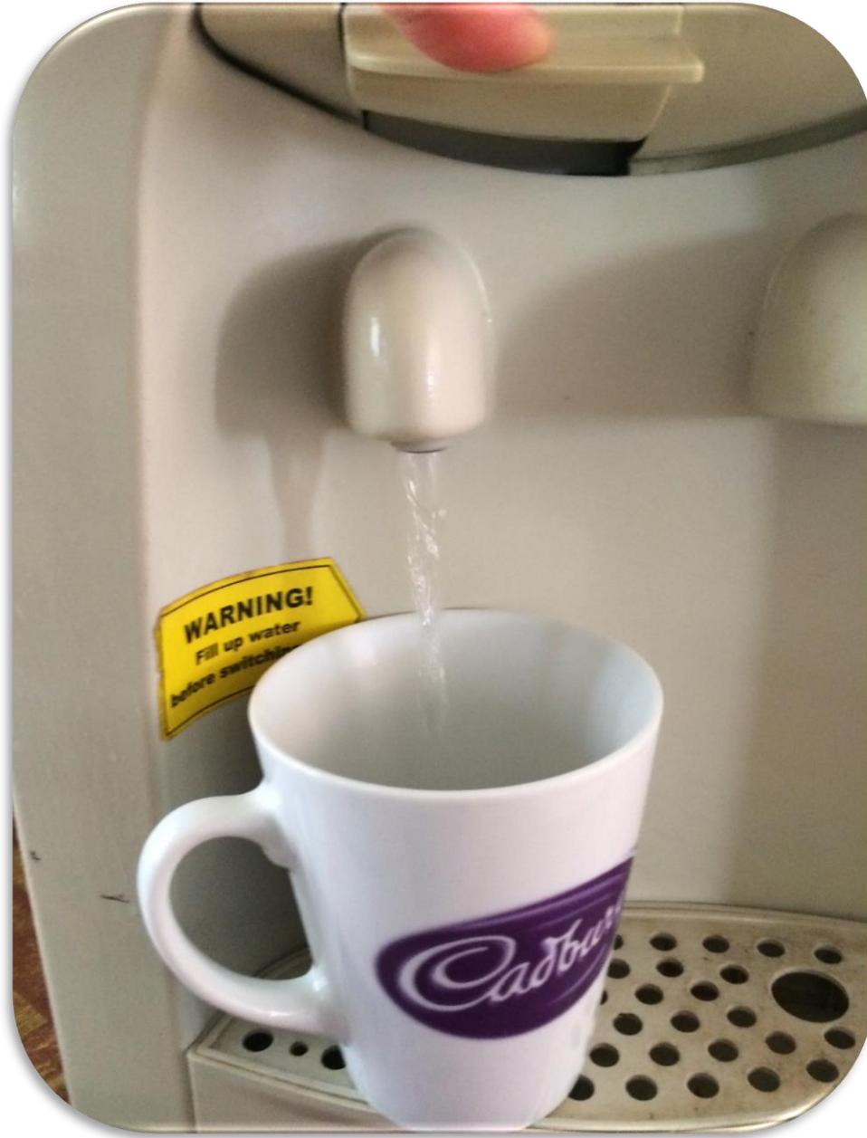
Replace bowl & filter and refill with water but **DO NOT turn on** until you have a steady flow of water from hot tap.
