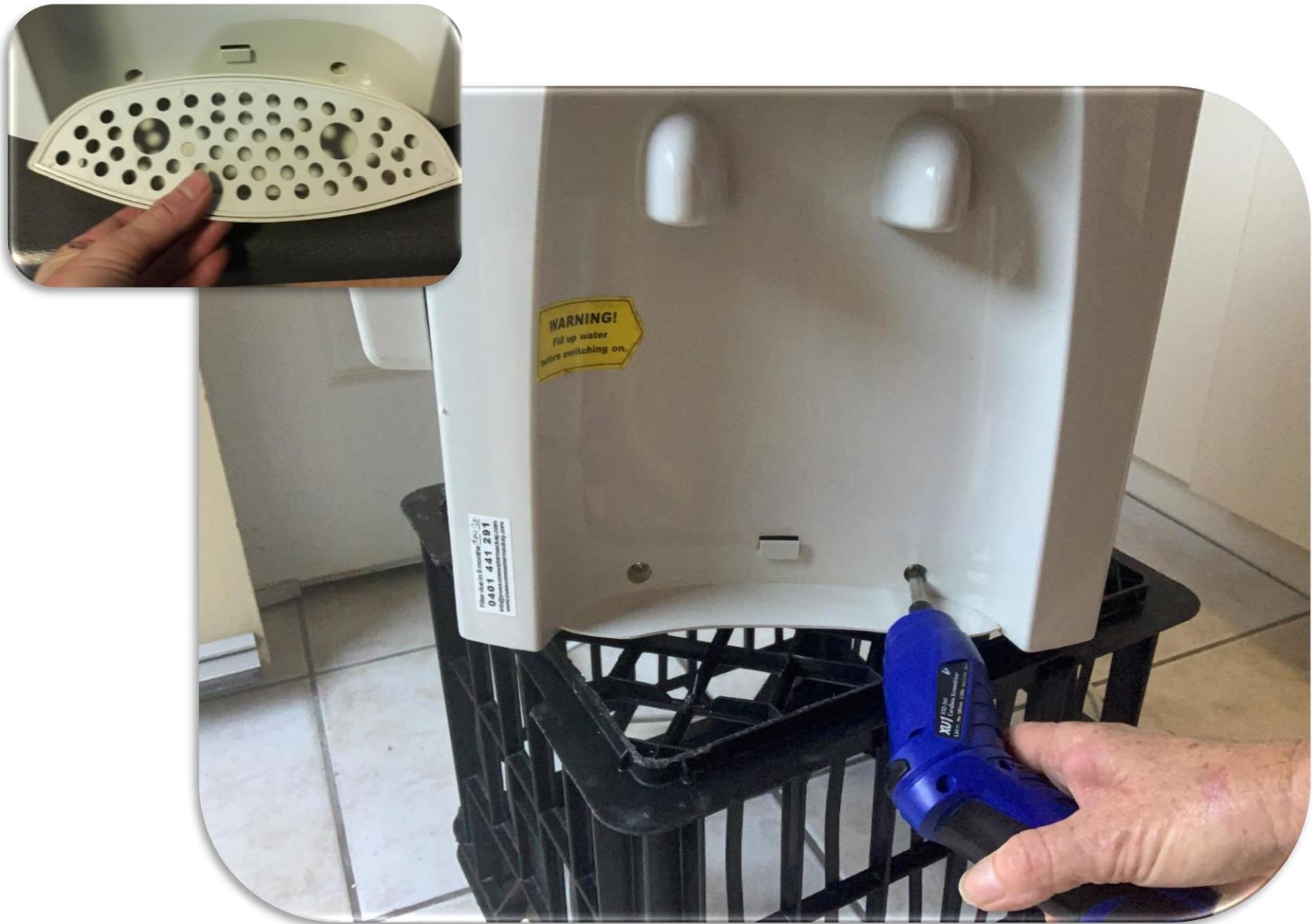
Remove drip tray & unscrew 2 x screws located behind drip tray.
