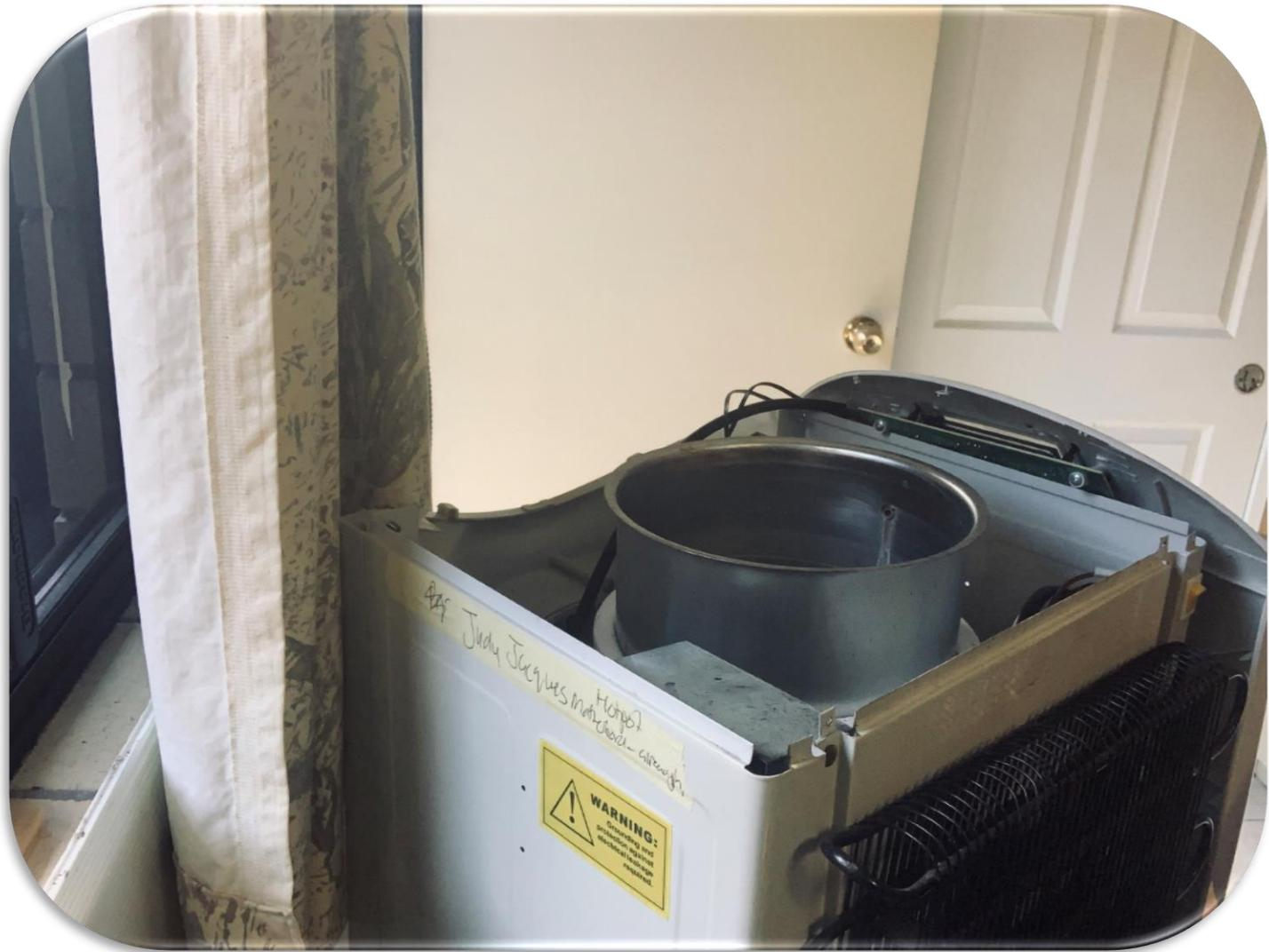
Remove top cover, hanging it on the side while ensuring that wires stays in tact
