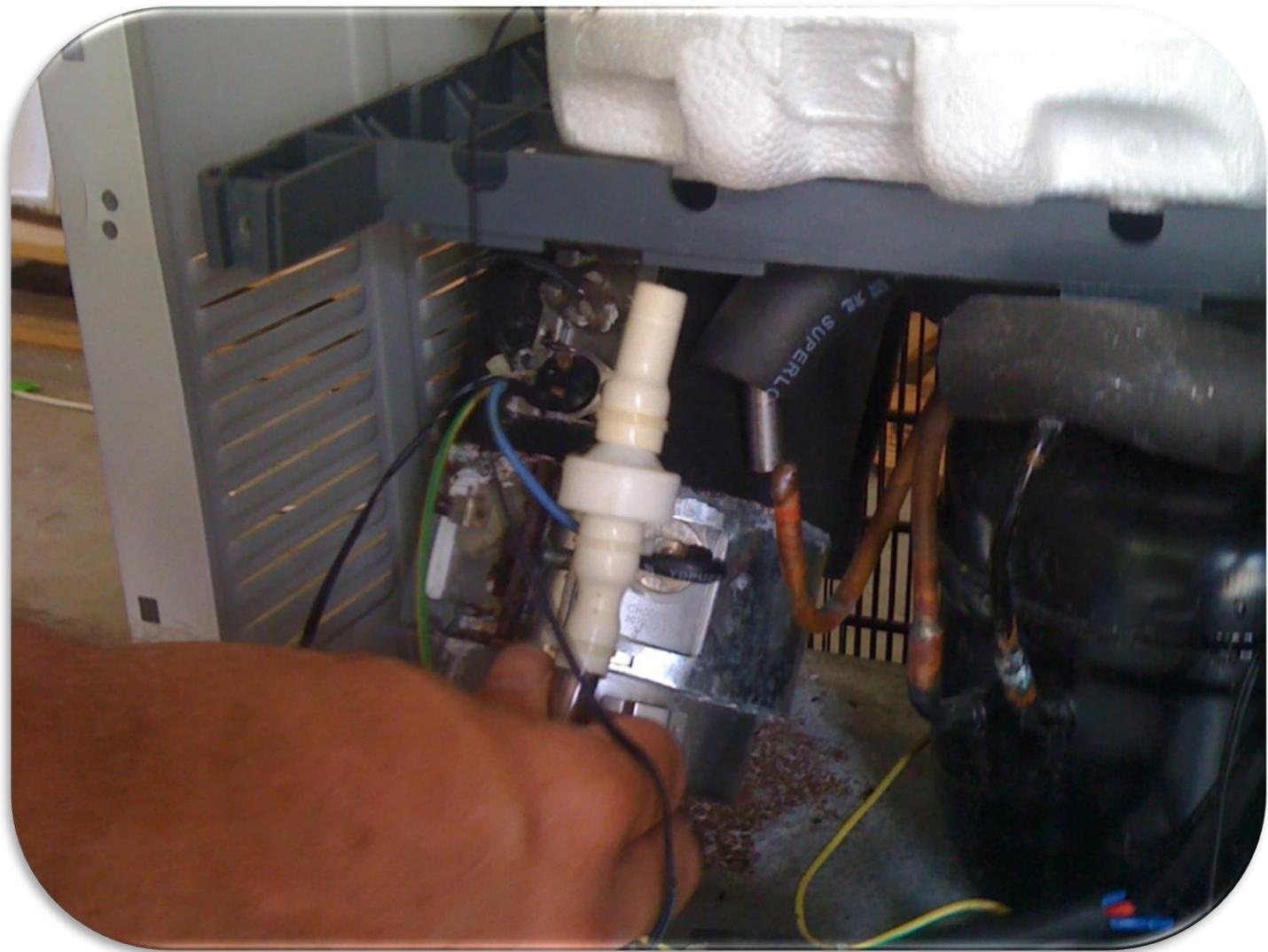
**Hot pot can now be removed by pulling out from the bottom. This can be a bit tricky and you'll need to try a few angles to get it out through the holes.**
