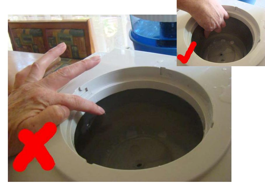
If the water tank is more than half way full it means the float valve is not locking
