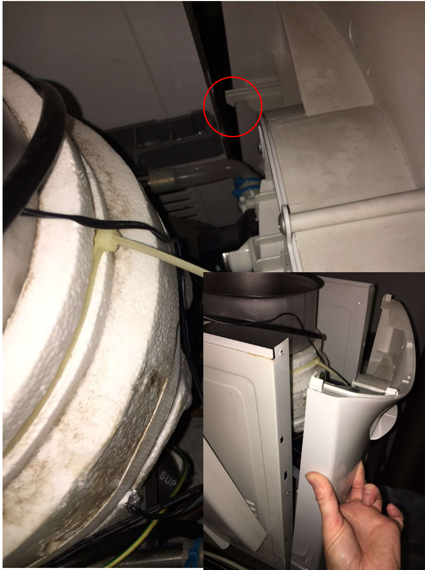
7. Unclip hooks securing the front cover the machine
