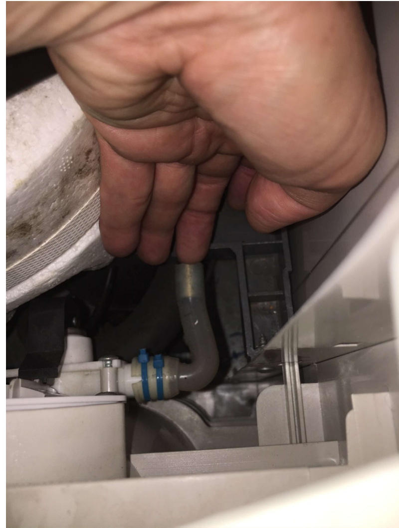
6. Use your name to push silicone tube off pipe – this could be tricky, just continue bit by bit
