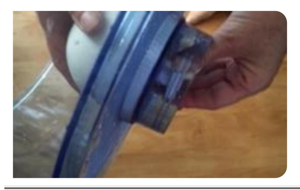
Use nut to screw back dome to top bowl - do not over tighten
