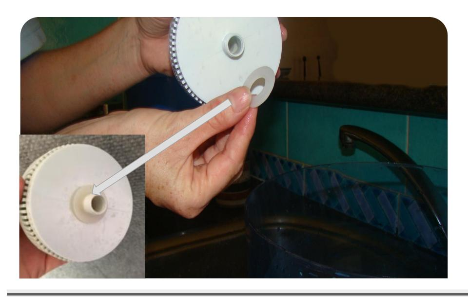
Check that the washer is in place at the bottom of the dome
