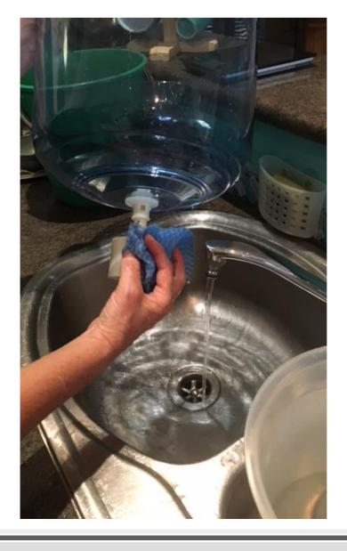
Rinse the float valve under running water and clean with a chux. You might need unscrew it from the bottom bowl if it is very dirty to clean it properly.
