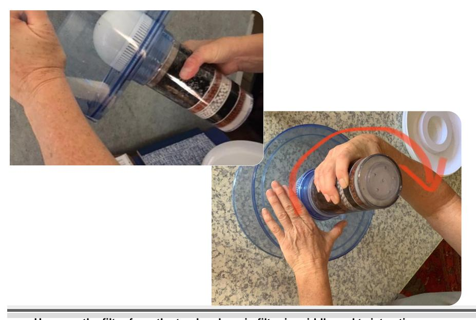
Unscrew the filter from the top bowl – grip filter in middle and twist anticlock wise, Be careful not to use too much force holding onto the top of the bowl as it might crack. A safer option is to put the bowl upside down on a flat surface and then unscrew the filter.
