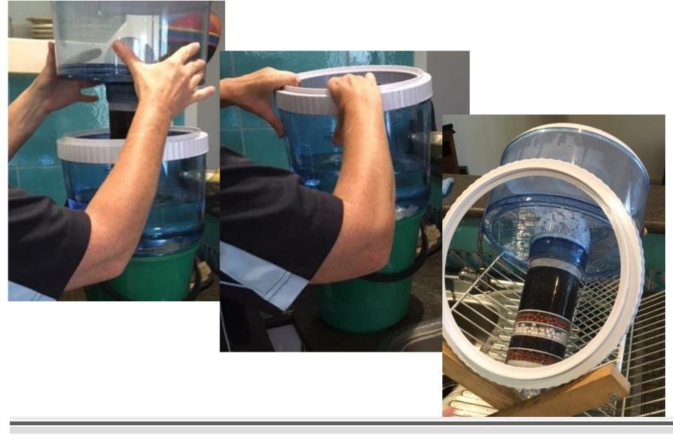
Remove Lid, lift top part of the bowl, remove white rim & put both in a secure spot.
