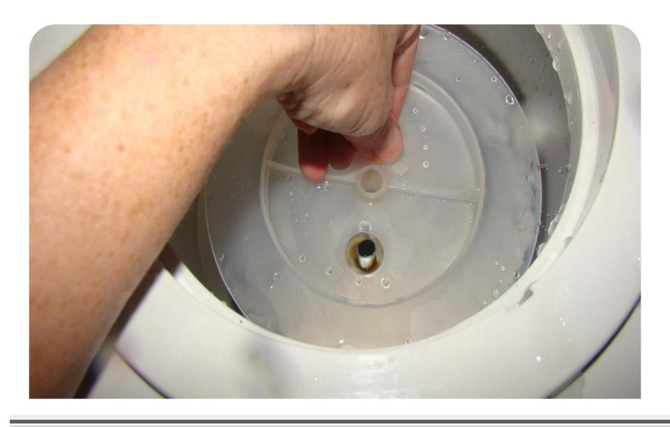
Return base plate by putting your finger through one hole and using the other hole to look through to find spindle.
