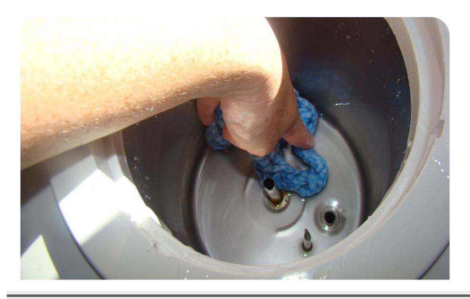
Use clean cloth to soak up last bit of water, and wipe tank clean Remember to also wipe down sides to remove any bio-film & calcium buildup. 6
