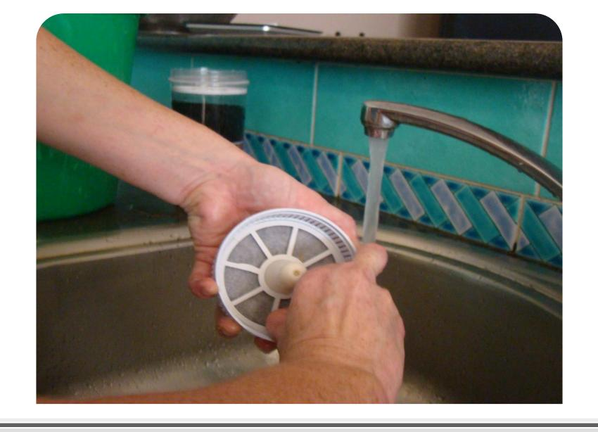
Pull out grid from dome and remove cloth filter
